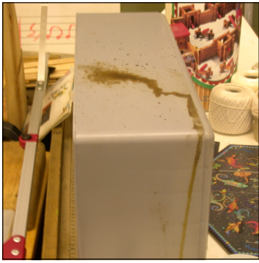
PCBs leaking on to a classroom tool box.
