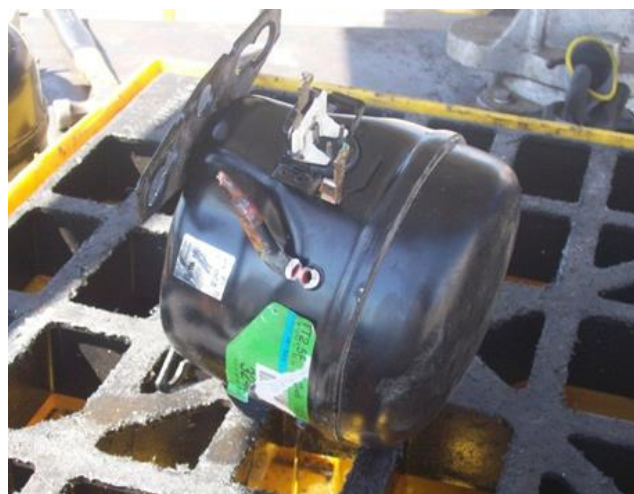
Figure 2: Compressor being drained of oil on a drain rack
