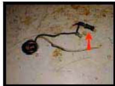
A chest freezer light with an in-line mercury switch.
