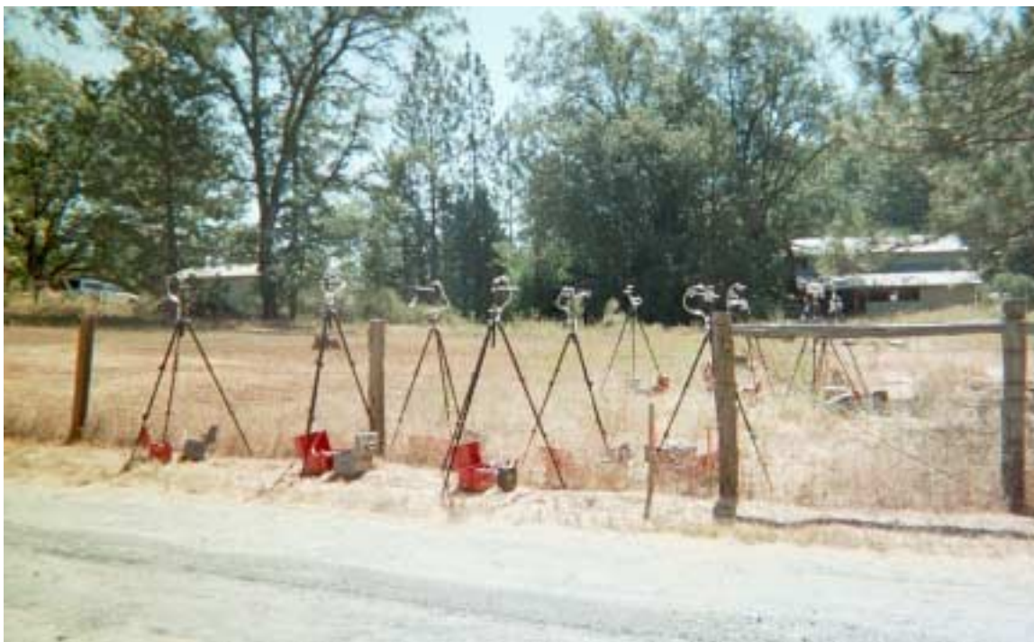
Figure A-4. Air samplers, located at various distances from the road along a transect perpendicular to the road.
