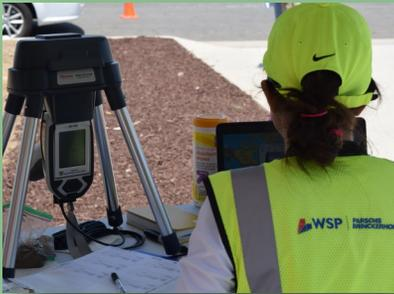
*Soil is being tested in the field with a reliable and calibrated XRF instrument and samples from each location are also being tested in a certified lab.*
