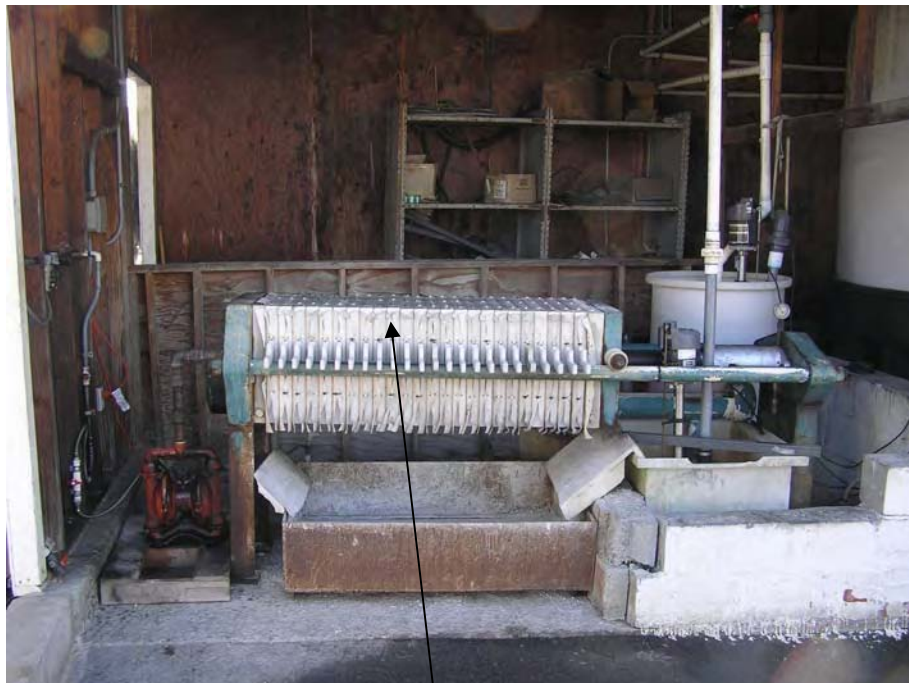
Another example of a filter press used to dry F006 waste
