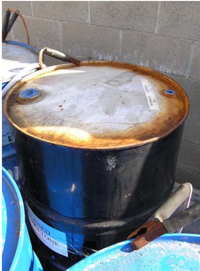
This photograph shows an inadequately labeled, and bulging, drum of waste acetone sitting next to the property line.
