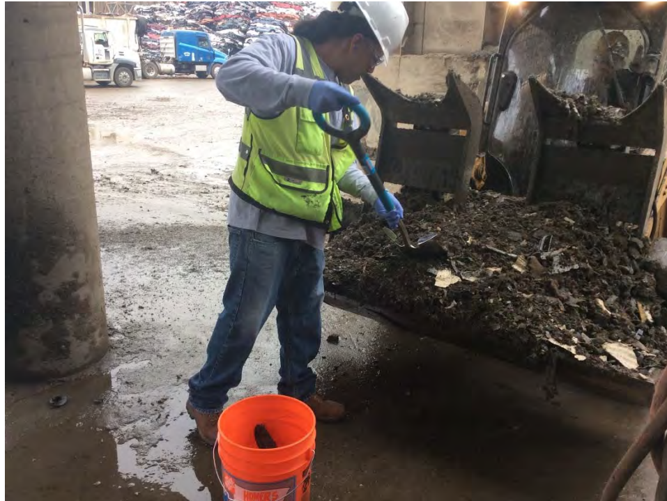
Photograph 23: Collection of an hourly sample of treated MSR. The treated MSR stockpile was cleared and the bucket of a skid-steer loader was positioned beneath the discharge stream for approximately one minute. A clean shovel was then used to transfer MSR from the loader to a clean 5-gal bucket.
