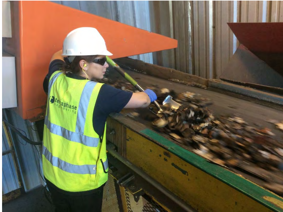
Photograph 17: Collection of an hourly MSR sample from the “oversize” untreated stream.
