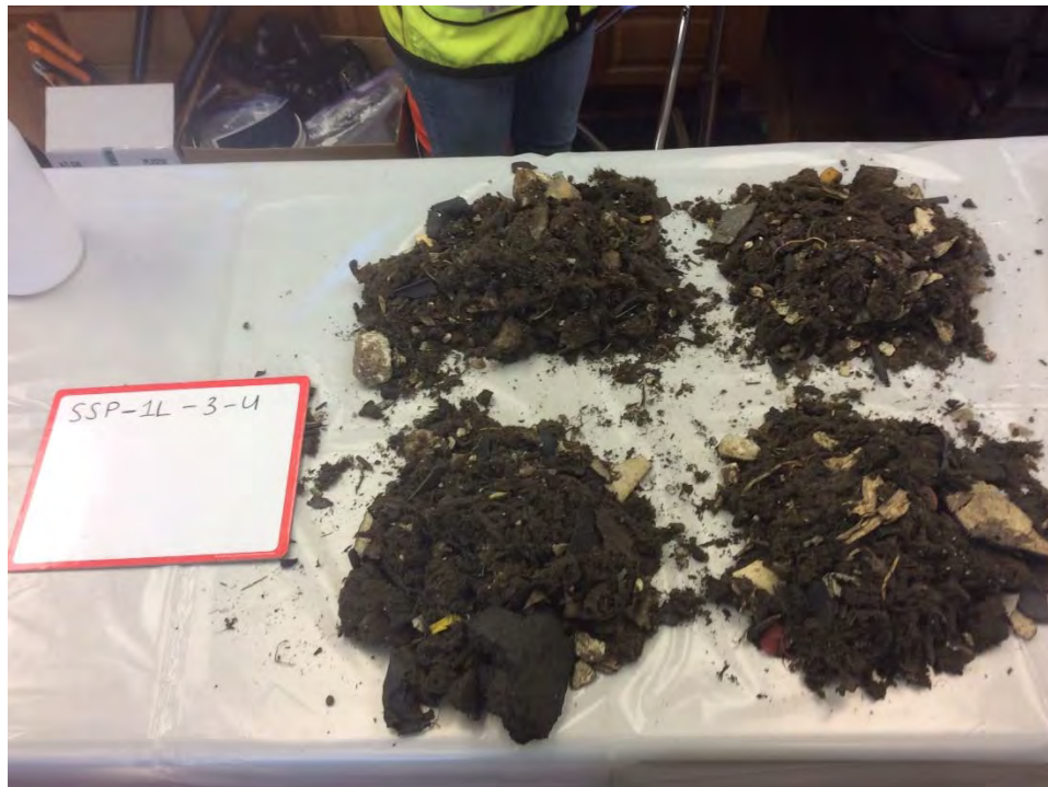
Photograph 24: MSR was collected into a 5-gallon bucket and placed onto clean plastic sheeting. Coning and quartering was performed.
