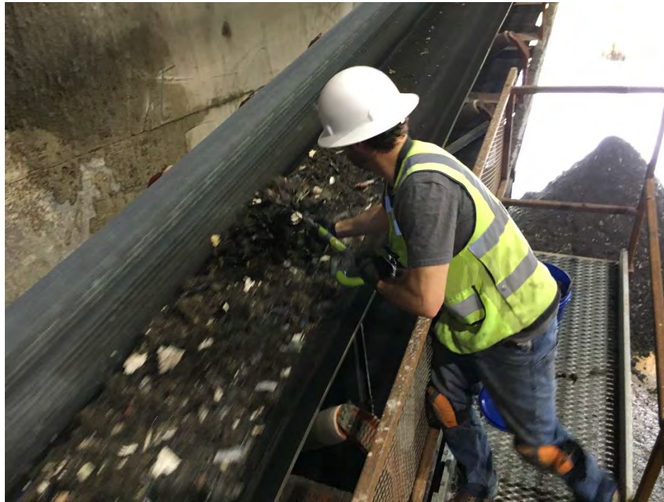
Photograph 11: Collection of a half- hourly sample of untreated MSR.
