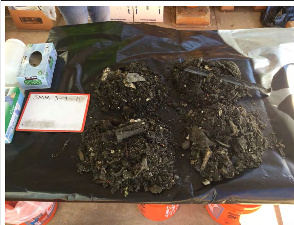
Photograph 19: MSR was collected into a 5-gallon bucket and placed onto clean plastic sheeting. Coning and quartering was performed.
