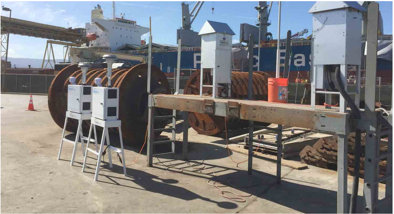
Photo No. 1 Sampling location SMM1. Equipment shown from right to left, TE-1000 PUF, TE-5170V, TE-Wilbur2.5, and TE-Wilbur10. A 6-Liter Summa canister (not pictured) was set up on the platform with the TE-1000 PUF and TE-5170V samplers. GilAir pumps are located behind this set-up. Also pictured is the freighter ship unloading bauxite in background.
