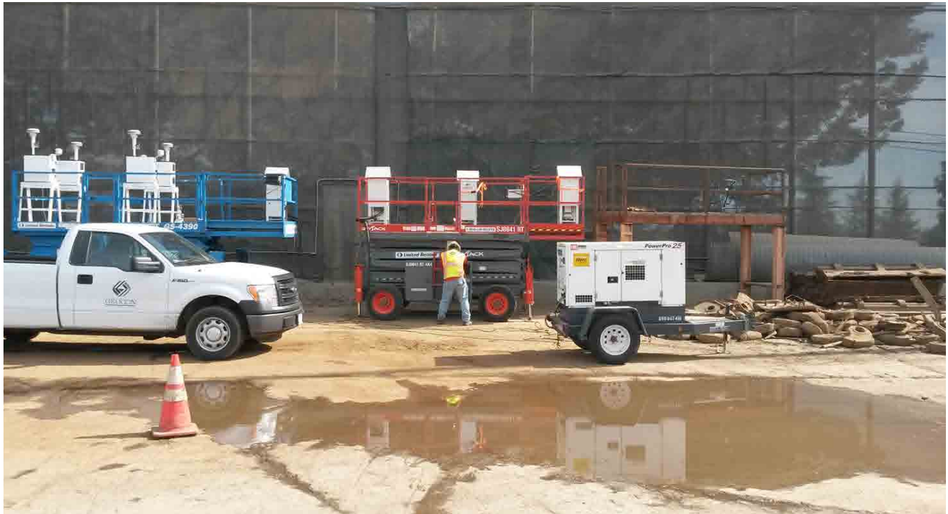
Photo No. 2 Sampling location SMM2 along with duplicate sample SMM5. During sample collection, scissor lifts were extended so that sample inlets were above the fabric-lined perimeter fence shown in the background.
