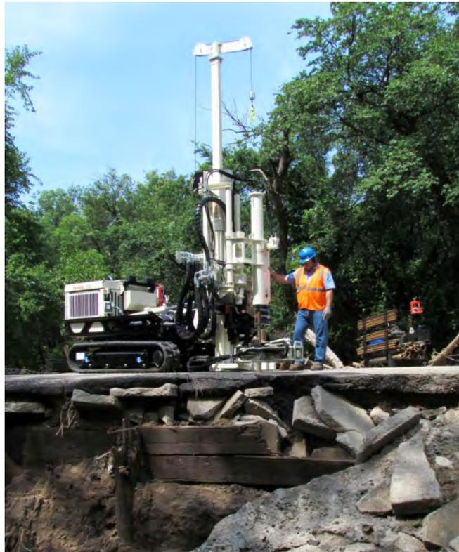
**Figure 4 Direct Push Rig** (Courtesy of Geoprobe® Systems)
