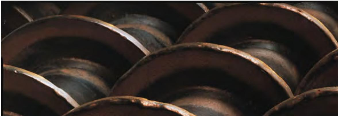
**Figure 2 Hollow Stem Auger Flight (Courtesy of Gregg Drilling)**
