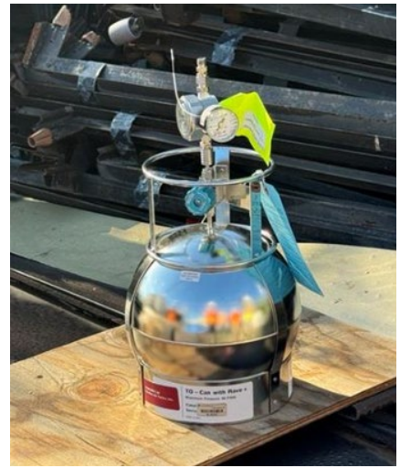
A canister set on site will capture vapor gas from the air for an 8-hour period.
